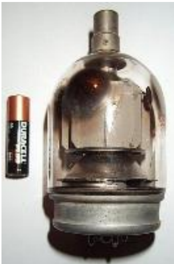
This valve measures 130x67mm overall
