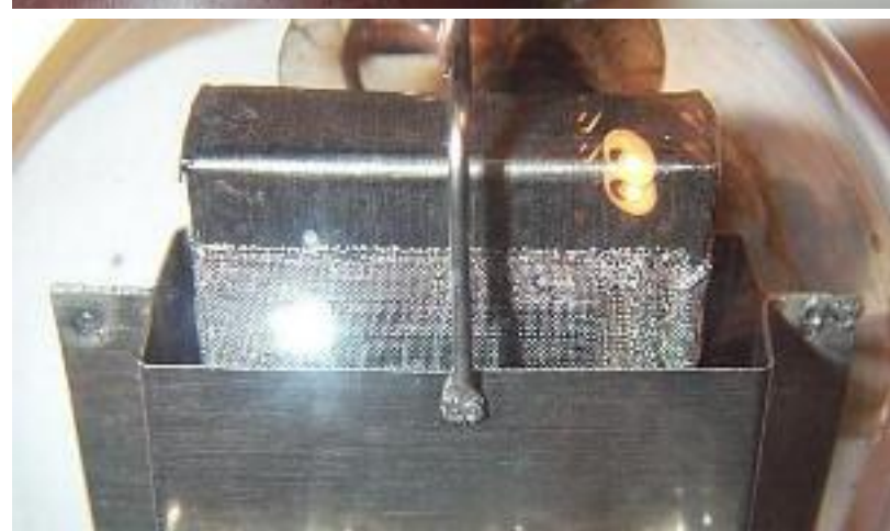
Anode connection is from the top connector. The anode connection plus G2 can be seen here.
