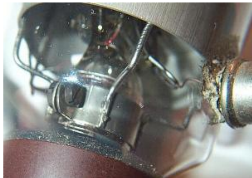
The base. The side connector connects to G1; G2 is connected to the metal ring at the top of the picture.
