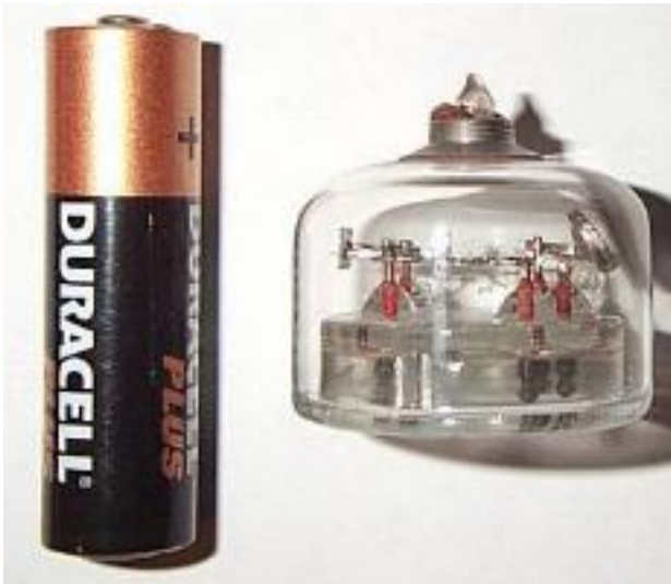
This valve measures 32x30mm overall and has a 5 pin base.
