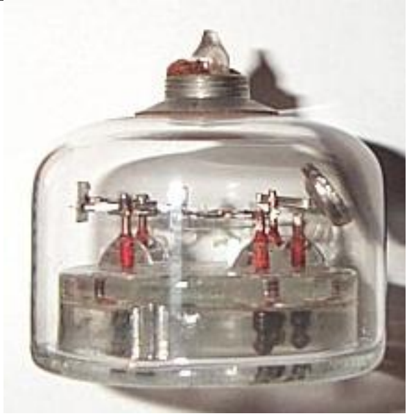
This valve measures 32x30mm overall and has a 5 pin base.
