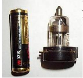
This valve measures 44x25mm overall and has 6 contacts around the base.
