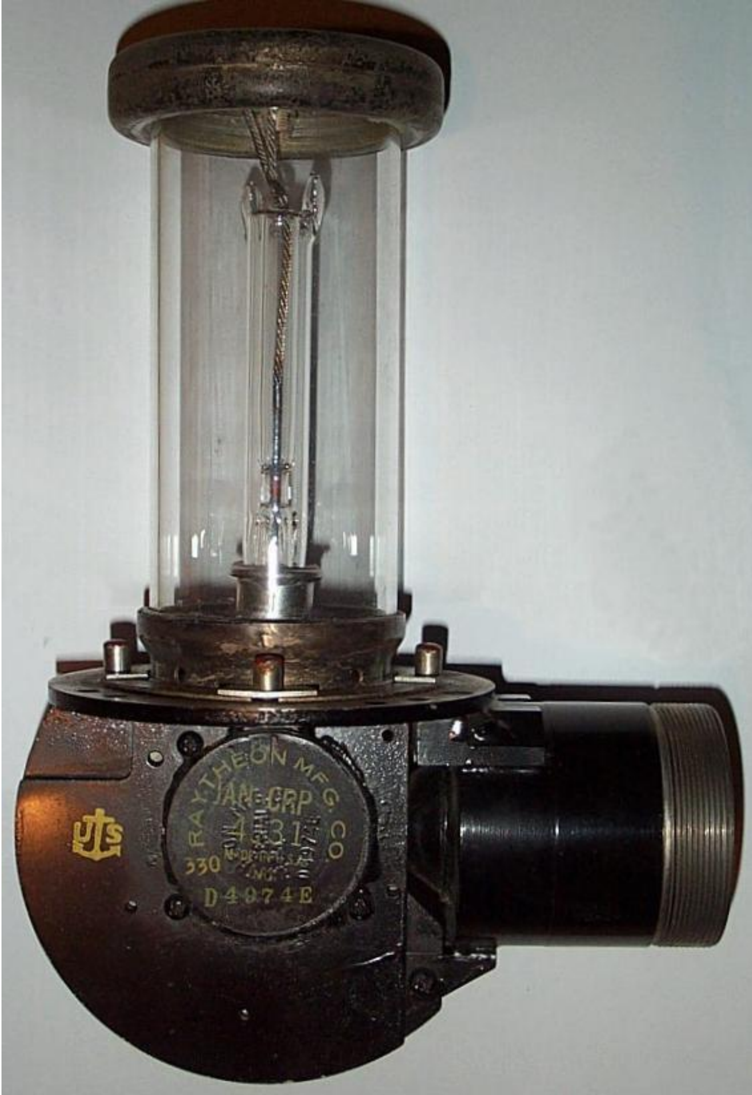
The 4J31 is one of a series of frequency variants (4J31 to 4J35). It was used in the AN/APN-19 beacon transponder.
