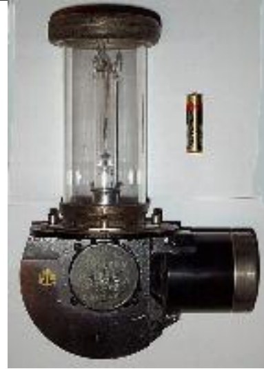
This magnetron measures 260x185x120mm overall.
