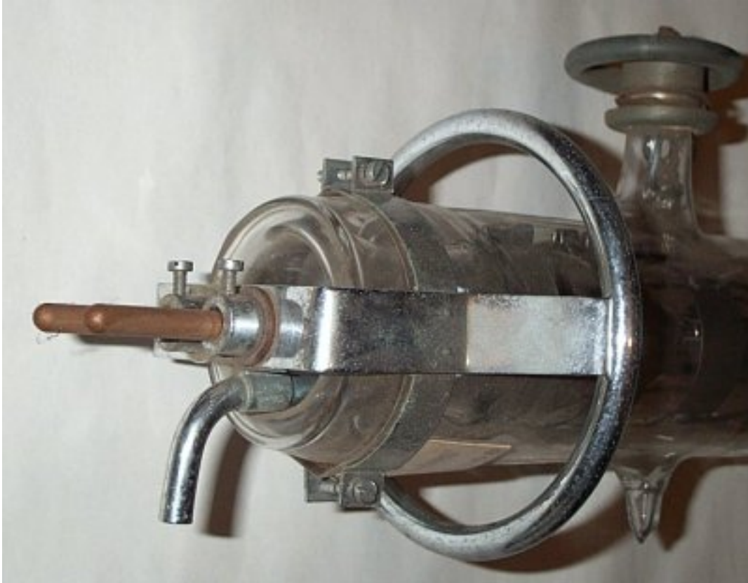
Above: Filament leads and air coolant connector. Below: Internal structure
