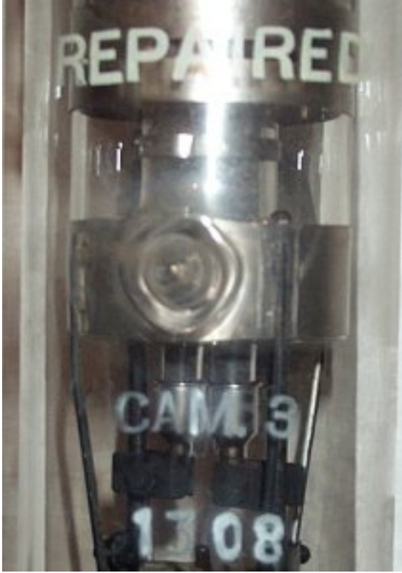
Markings indicate this valve has been repaired. Additionally, markings indicate that a filament voltage of 17.8V gives 7A emission at 90% saturation. The serial number is 1308.
