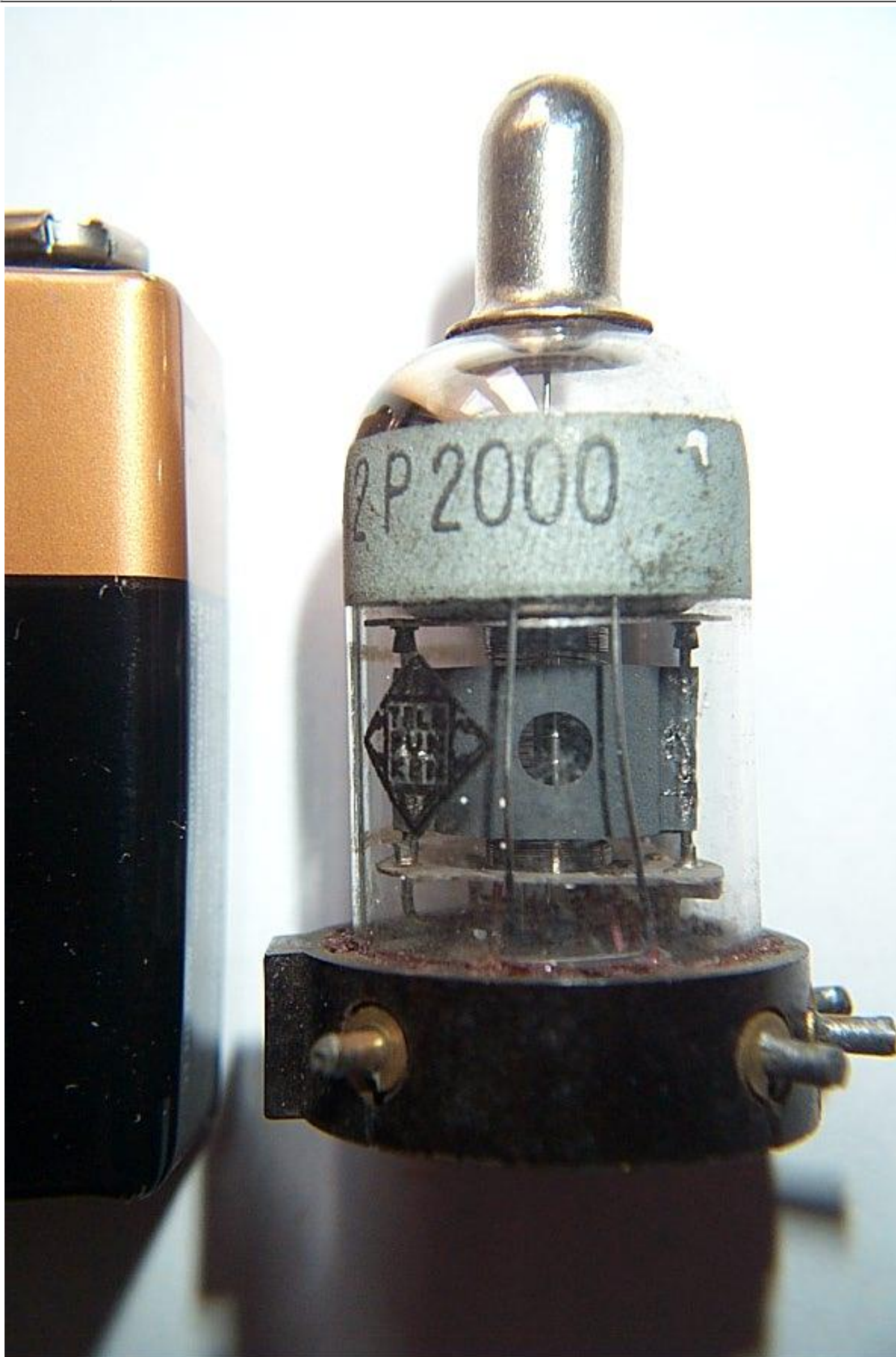
RV12P2000 pentode, 12.6V/70mA heater, 250V anode.
